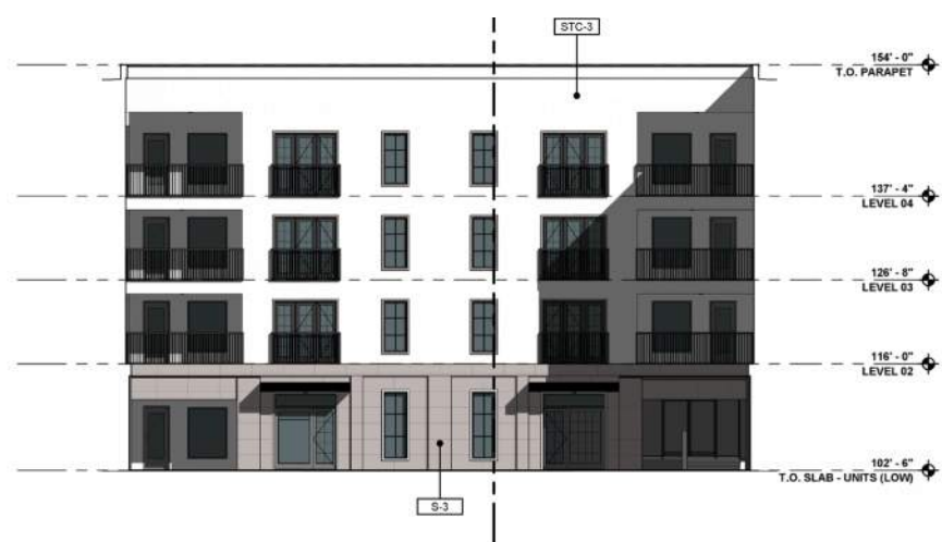
08 COURTYARD EAST ELEVATION SCALE: 3/32" = 1'-0" REF: 01 / A201
