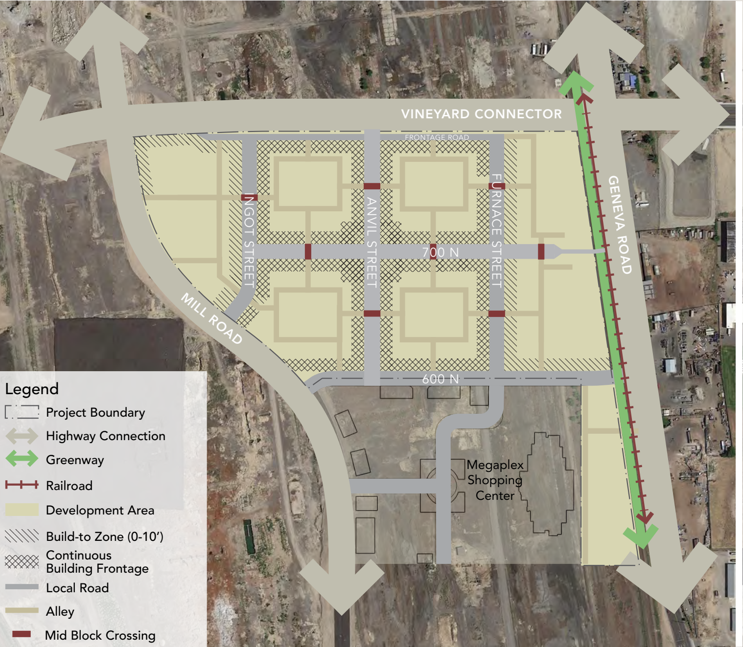
Figure 2.3 - Building Frontage and Build-to Zone
