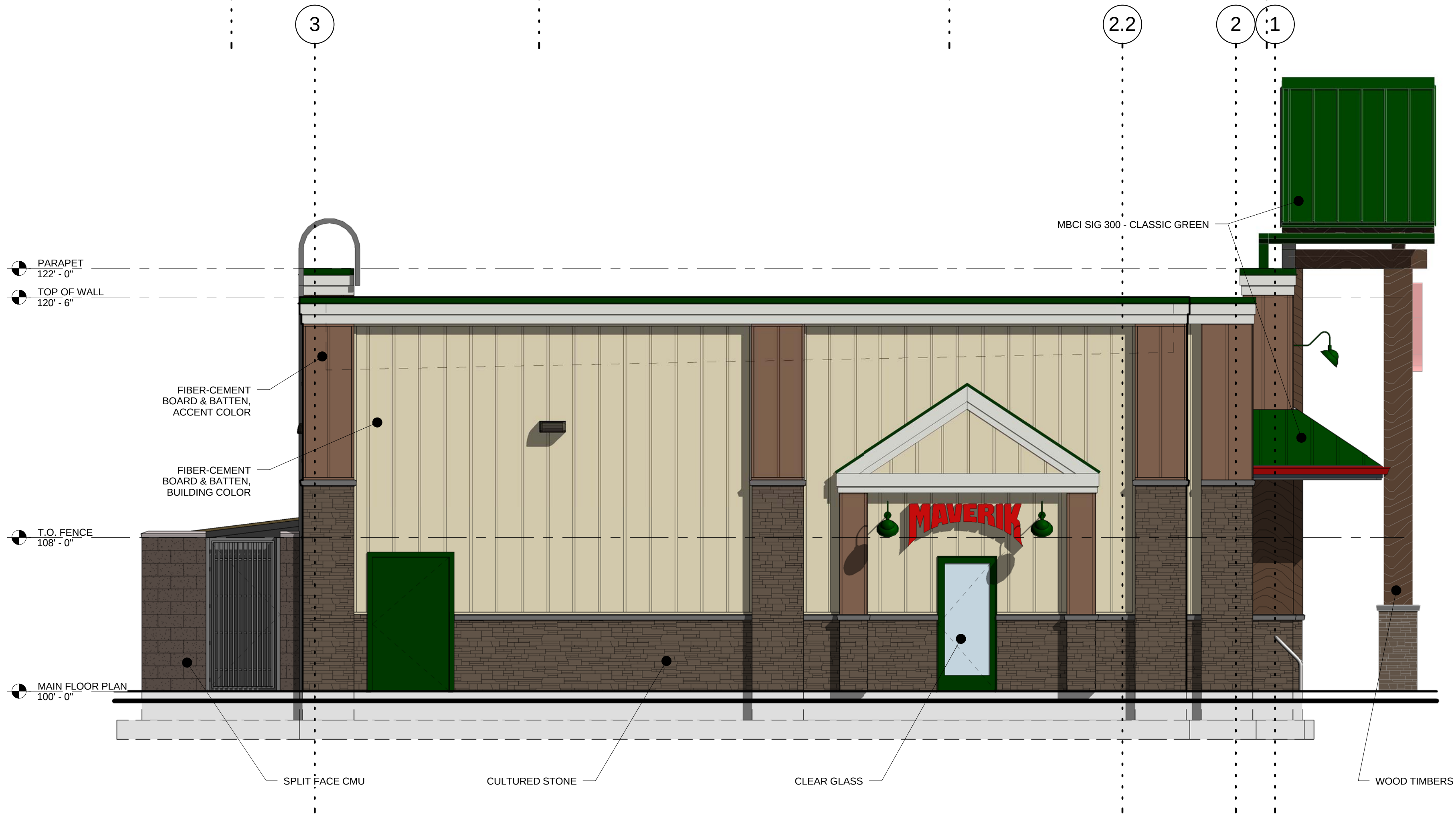
2 LEFT ELEVATION - COLORED A-2.1C scale: 1/4" = 1'-0"
