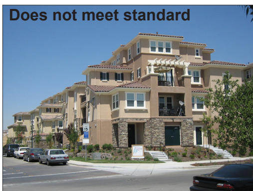
Figure 5.6.2.i and 5.6.2.j: Roofs should be simple in form, the building on the left does not meet this standard as the roof massing is overly complex while the building on the right has a more ordered variety in roof form.
