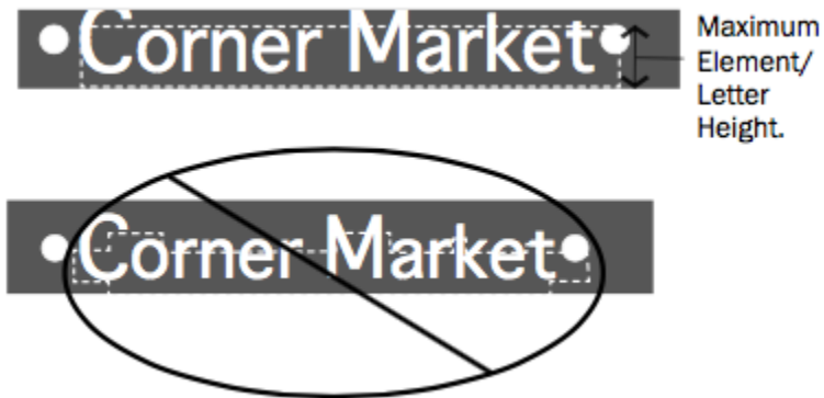
Figure: Measuring Wall Signs
