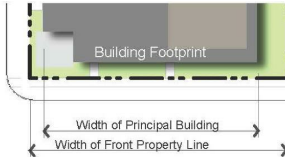
Figure 3.10.020(2). Measuring Front Property Line Coverage
